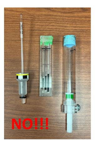
Depth gauges DO NOT go in the instrument.
