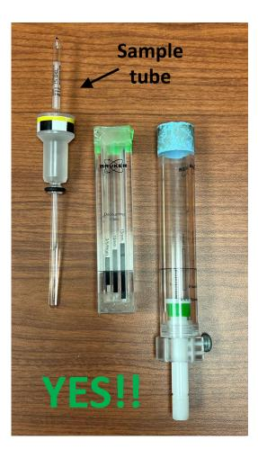
Sample tube inserted in spinner and set properly in the depth gauge
